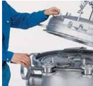
3. Open the cover aided by spring-assisted mechanism.
